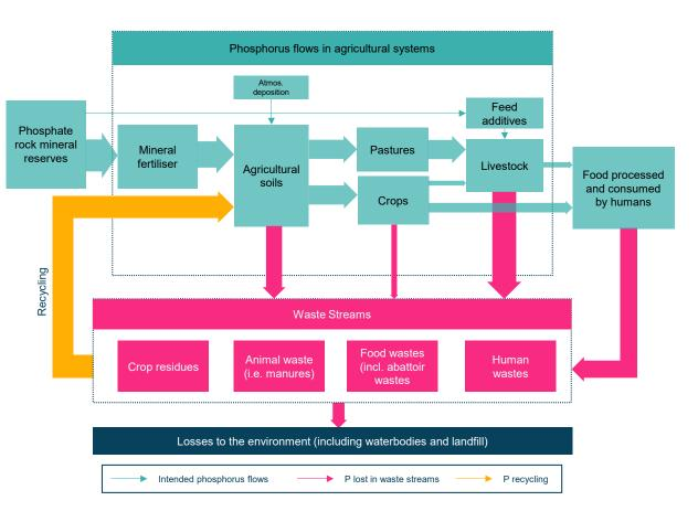
**Figure 4.2** A conceptualisation of the phosphorus (P) flows to, within and out of agricultural systems (not including aquaculture and forestry). The width of arrows is proportional to the amount of P estimated in each flow and is based on data from Chen and Graedel (2016). However, wide variation not only exists between nations/farms but also within the flows reported in the literature (particularly for P losses from manure and soils).
